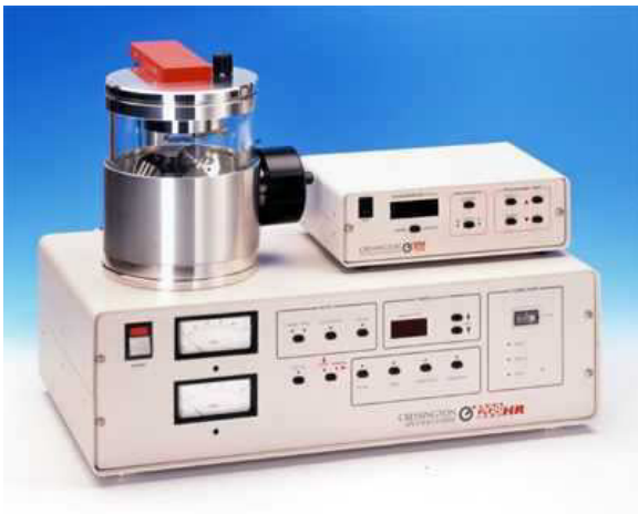
Fig 1. 208HR with thickness measurement
